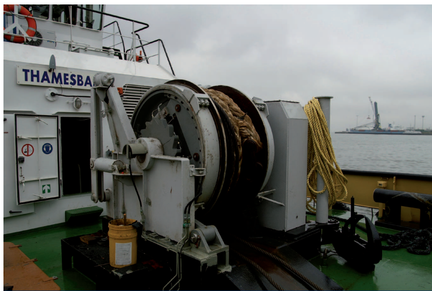
Fig. 8: The upgraded SafeWinch on the Thamesbank of Smit showing the new twin shoe clutch and the ratchet arrangement.
