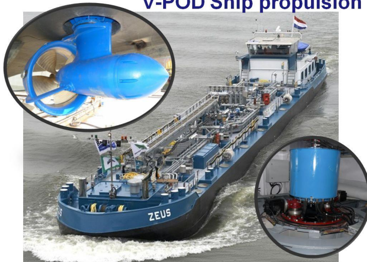
First vessel with V-POD and conventional slipring system
