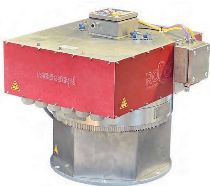
Detailed view of RoCo with at half height the rolling contact box, below the support frame and on top the connector box.
