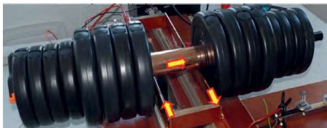
Picture of first prototype with rolling contacts with high pressure and current flow by arrows.
