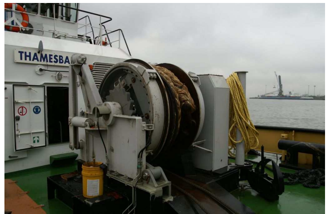
Fig. 8 : The upgraded SafeWinch on the Thamesbank of Smit showing the new twin shoe clutch and the ratchet arrangement.
