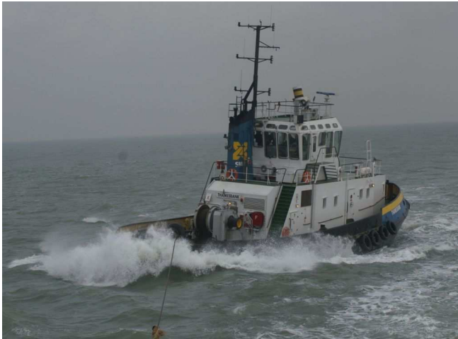
Fig. 10 : Dynamic sea tests, SafeWinch cuts off peak loads and prevents slack wire
