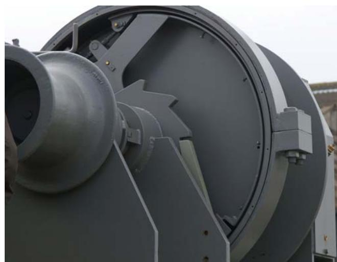
Fig. 10 : Installed ratchet on SafeWinch
